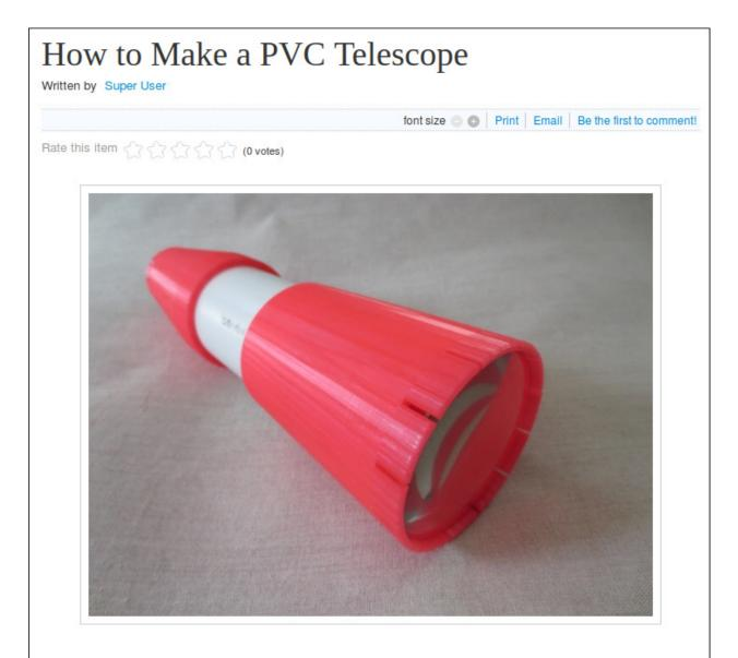
Placing any two convex lenses (with different focal lengths) a distance apart will create an up-side-down magnified image of far away objects.
